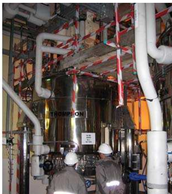
Filtering a crystallised solid in a large manufacturing plant. The plant has four of these huge filtration vessels running in parallel for one batch.
