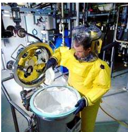
Filtering a crystallised product in a small pilot plant
