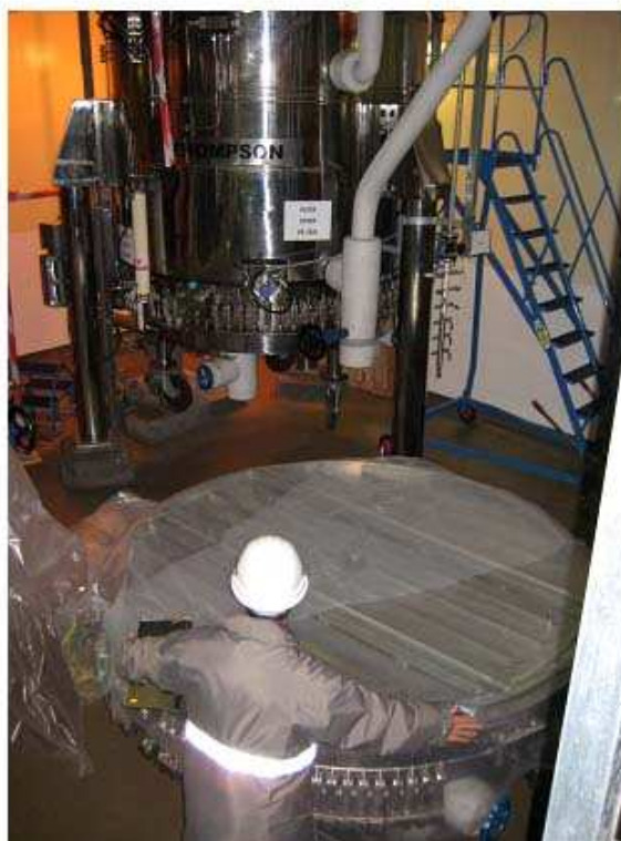
Filtering a crystallised solid in a large manufacturing plant. The plant has four of these huge filtration vessels running in parallel for one batch.
